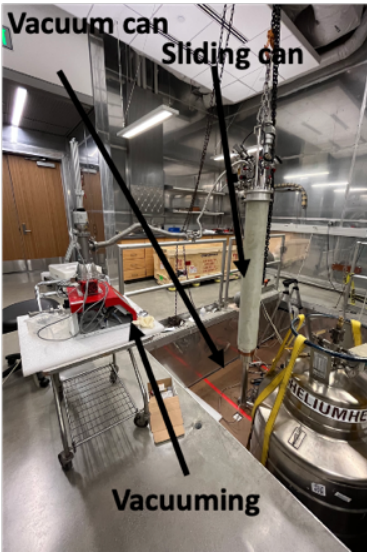
Figure 62. Main dilution refrigerator used in this thesis: (a) vacuum preparation of the cylinder before loading the sample to fridge chamber. (b) Cylinder inside the fridge chamber. (c) Cylinder unloading from the chamber.
