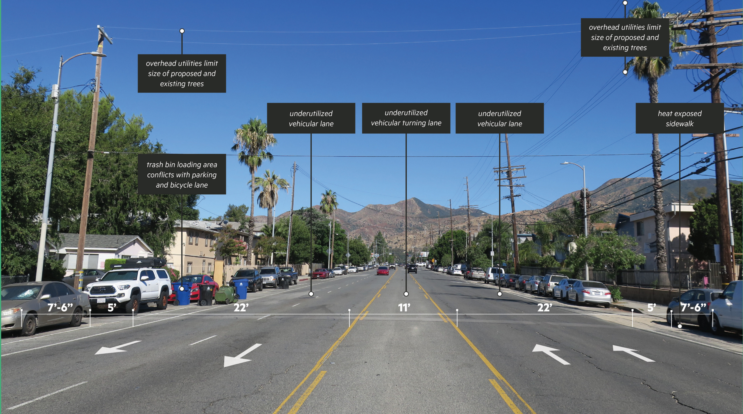
Figure 23. Foothill Boulevard and Astoria Street, challenges and opportunities Credit: Stoss Landscape Urbanism
