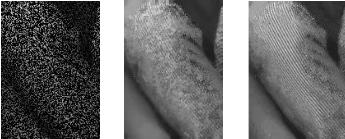
(a) damaged image- 35% of the pixels removed (b) local TV inpainting- PSNR 22.6530 (c) our method's result- PSNR 24.1266
