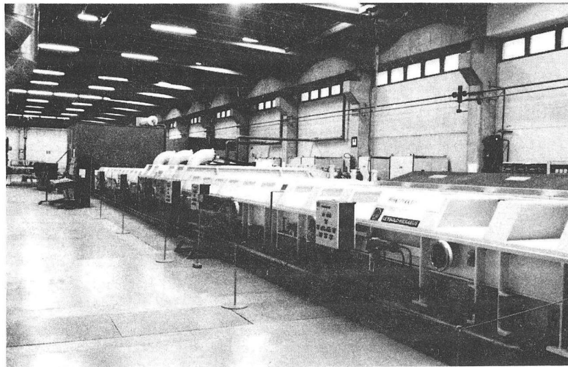
Figure 7. Load lock in-line sputter system for glass coating.
