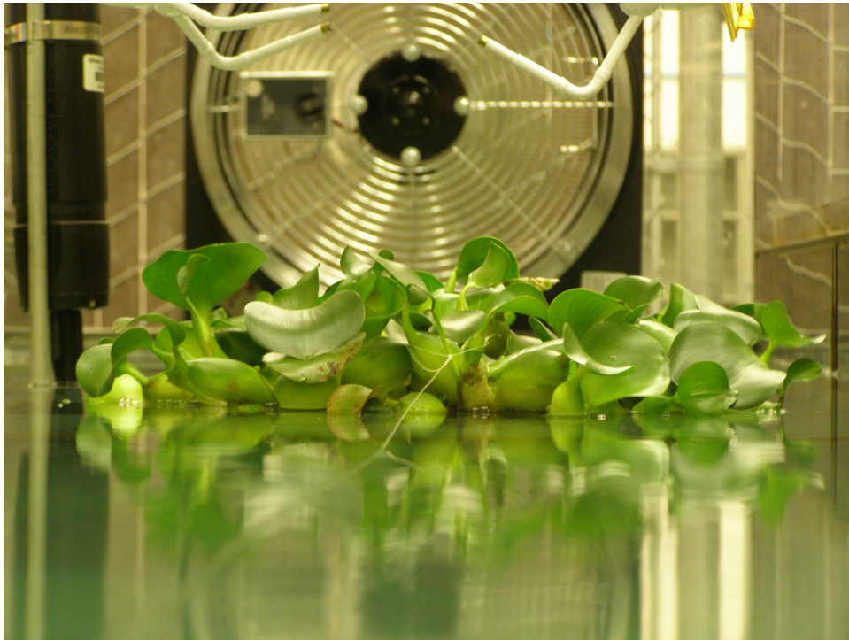
Figure 4.3: Photograph showing vegetation raft floating in wind tunnel, taken looking downwind. Outward-blowing fan is seen at far end of photograph and sonic anemometer is seen near top of photo.
