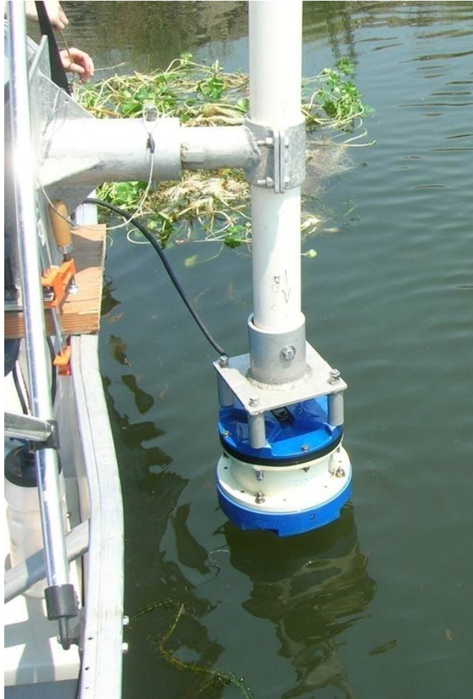
Figure 5.6: Photograph of ADCP setup for field experiment on August 1, 2008. The instrument was mounted at mid-length of the boat, off the starboard gunnel; the transducer head was deployed facing downward, toward the channel bed. During data collection, the transducer head was positioned 0.1 m below the water surface.
