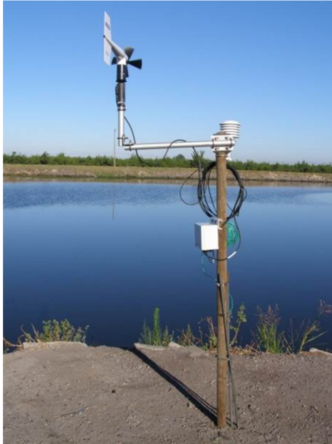
Figure 5.5: Photograph of anemometer setup for field experiment on August 1, 2008. Aerovane is shown mounted on upper left of frame and datalogger is shown mounted on center post. Photograph taken looking west across Bishop Cut.
