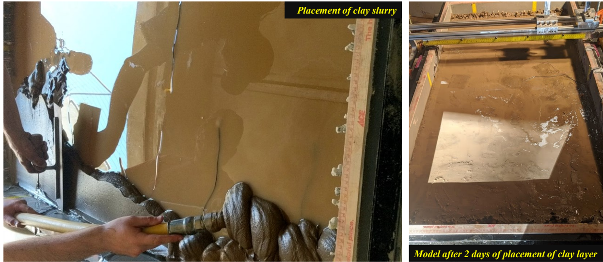
Figure 28. Placement of clay slurry in the model.
