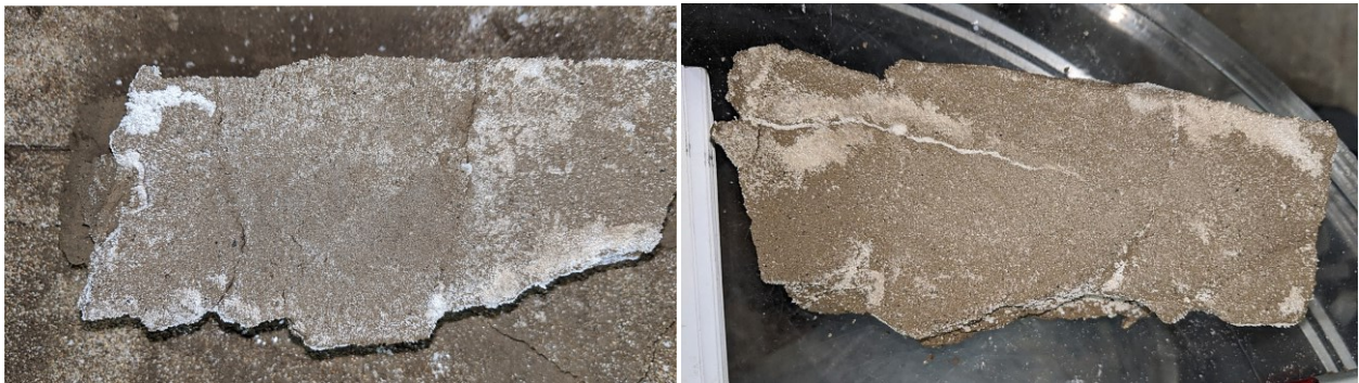
Figure 53. A view of the bottom of the clay layer showing presence of cracks.
