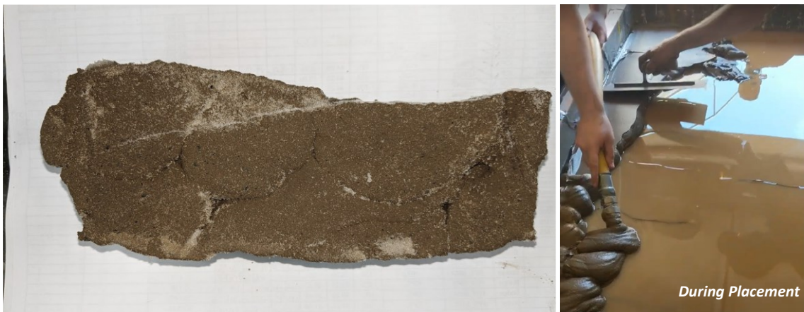
Figure 54. The bottom of the clay layer (on left) can be seen in clumps, like the way it was placed in the model (right).
