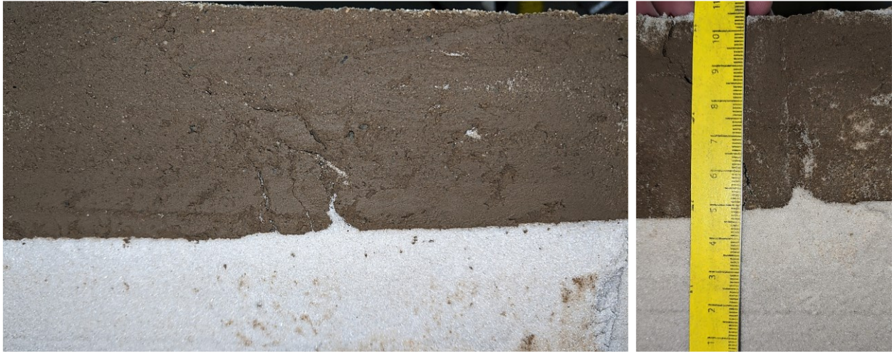
Figure 55. Ejecta observed below the clay layer
