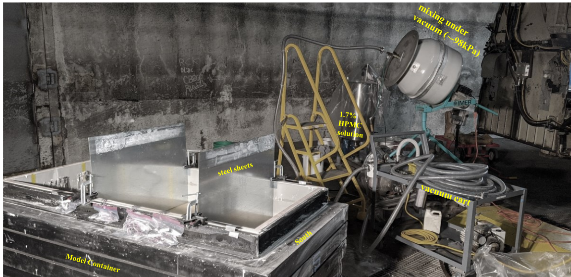
Figure 26. Setup for placing the loose sand layer as slurry.
