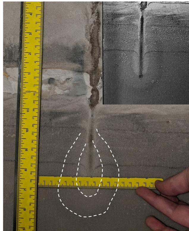
Figure 59. Cross-section view of Pile 1 after pile load test PLT_2 .
