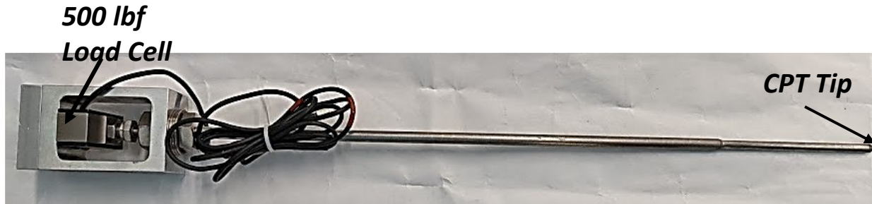
Figure 18. 6mm LEAP centrifuge cone penetration test (CPT) probe.
