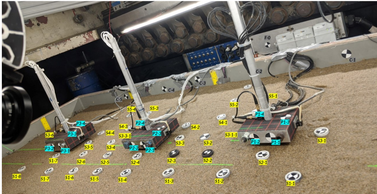
Figure 44. Camera target markers placed on soil, pile, model container, and centrifuge bucket.
