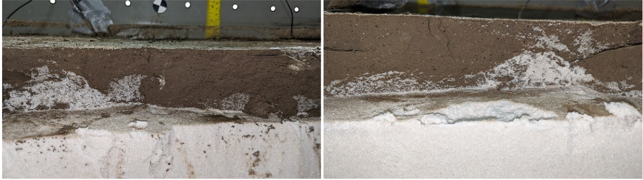
Figure 52. Cross-section view of the model showing movement of sand grains inside the clay layer from the soil beneath.
