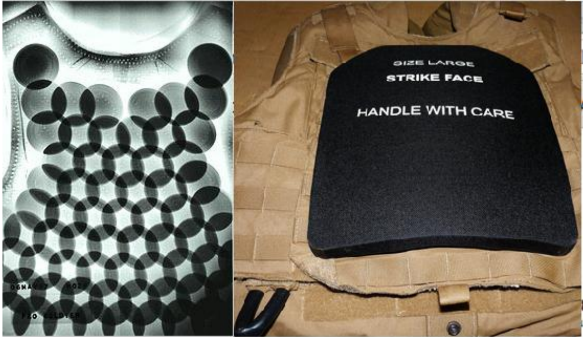
Figure 1.1 A comparison of the scale armor of Dragonskin (left) to the SAPI plate of the Interceptor Armor (right). Note the warning on the SAPI plate suggesting a material specialized for projectile impact (it cannot be dropped).
