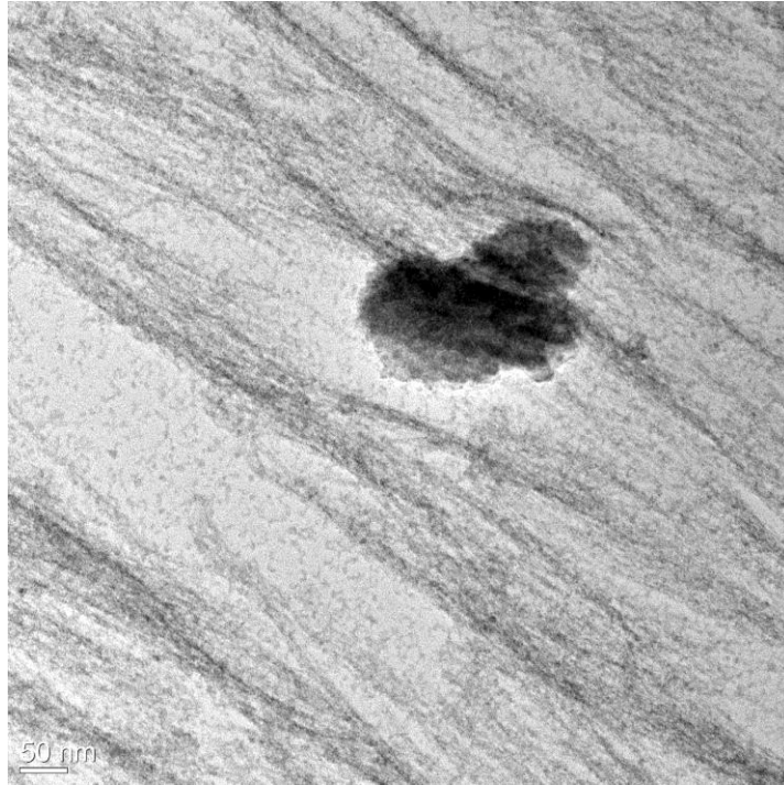
Figure 3.10 Mineral particles aggregate at the two sides of the same site of an organic fiber.
