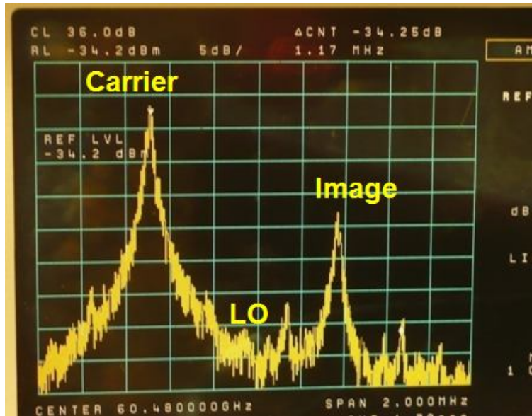
Fig. 4.26. The transmitter output spectrum of a single-tone test, this shows the carrier signal, the image tone, and the LO leakage tone.
