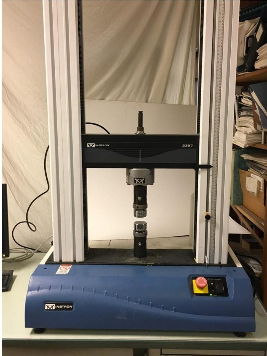
Figure 14 Quasi Static mechanical testing machine (Instron Model 3367).
