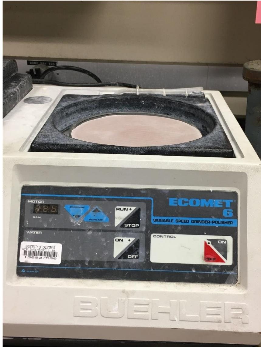
Figure 19 Ecomet 6 was used for polishing using the SiC papers and polishing cloth.
