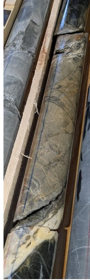
Figure. 4. Core photo of E2-AML at ~187 feet deep, showing some open portions of a highly fractured interval.
