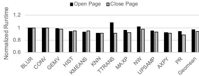
Figure 6.8: The normalized runtime of an ideal DRAM without refresh for both open page and close page policies over the DRAM with actual HBM timing.
