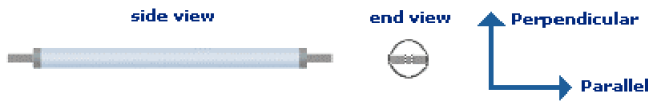
Fig. 4. A 300 mm Long Commercial HTS lead showing Field Directions Parallel (preferred) and Perpendicular (not preferred) to the Flat Face of the BSCCO Tape that is inside the HTS Lead.
