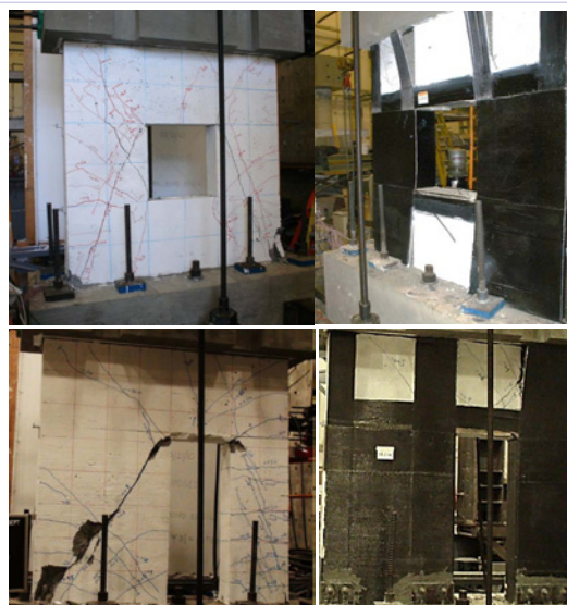
Figure 9: Failure modes of as-built and retrofitted wall with opening specimens.
