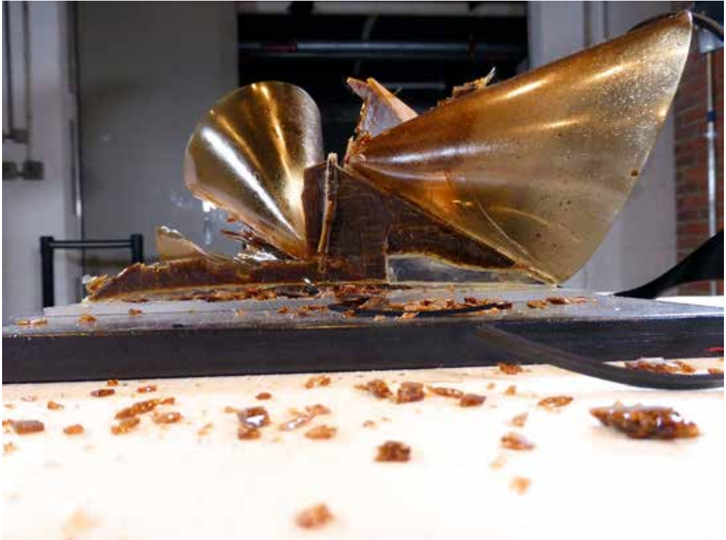
Figure 2.6. Naum Gabo artwork in cellulose acetate or cellulose nitrate. The circular relief (1925–1928) and other works have undergone autocatalytic degradation, resulting in the sculpture disintegrating on display. The sculpture shown here is Construction in Space: Two Cones , 1927, Philadelphia Museum of Art. In this example, inherent vice destroys the artwork without the need for human agency. (Image courtesy of Luke Barley, http://architizer.com/blog/naum-gabo-plastic-sculpture-decay/ )
