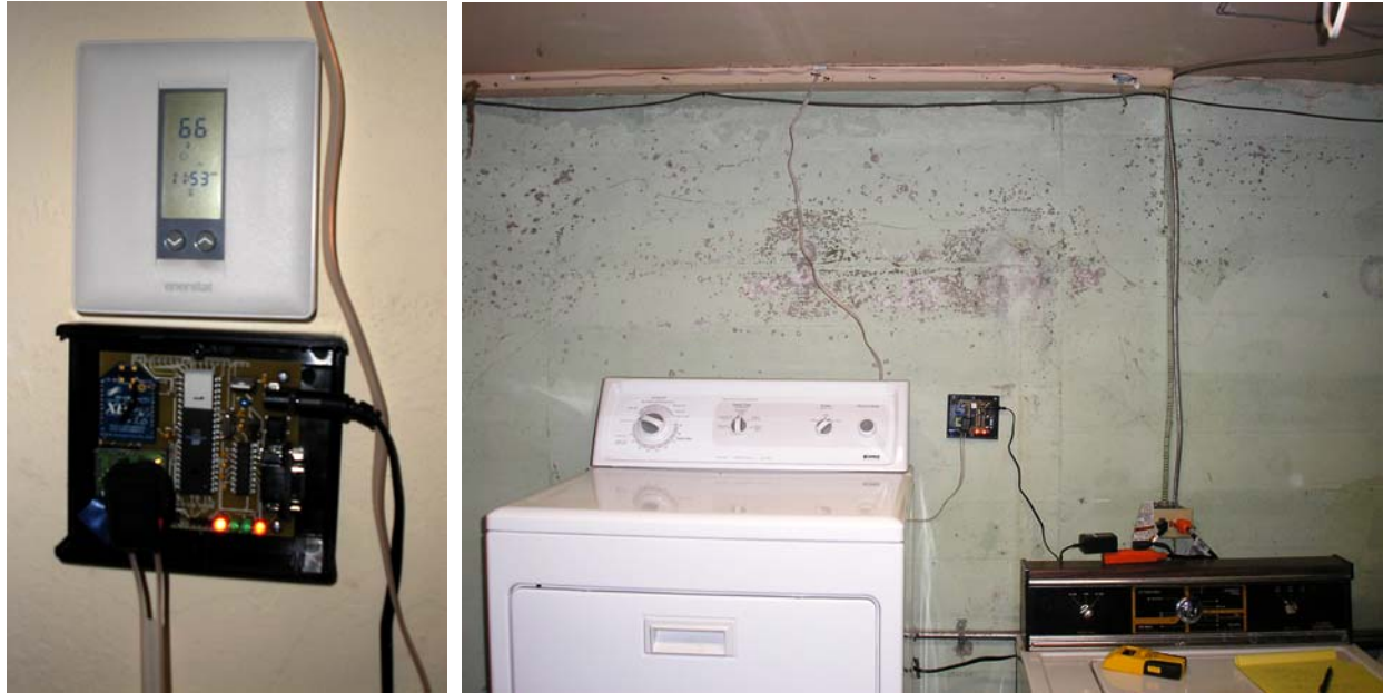
a) b) Figure 10.5. a) Data logger mounted below existing thermostat; b) Data logger mounted in basement next to washing machine, seen with dipole antenna mounted near ceiling
