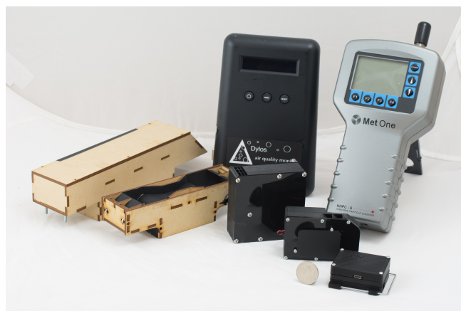
Figure 2. Design iterations, from initial cardboard mock-up to current 3D printed wrist worn prototype. The large commercial Dylos & MetOne are shown for comparison.
