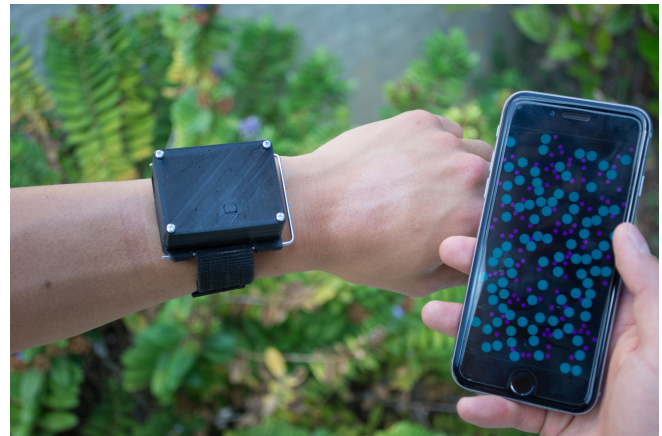
Figure 1. The small wrist-worn MyPart sensor and optional accompanying smartphone visualization and data logging app.
