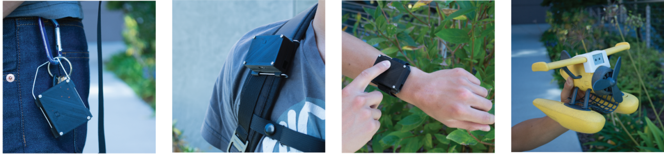
Figure 8. Highlighting the flexibility of the MyPart design form factor by demonstrating the ease of adapting it to function as (from left to right): a carabiner, a backpack strap, a wristwatch, and even embedded into a toy airplane
