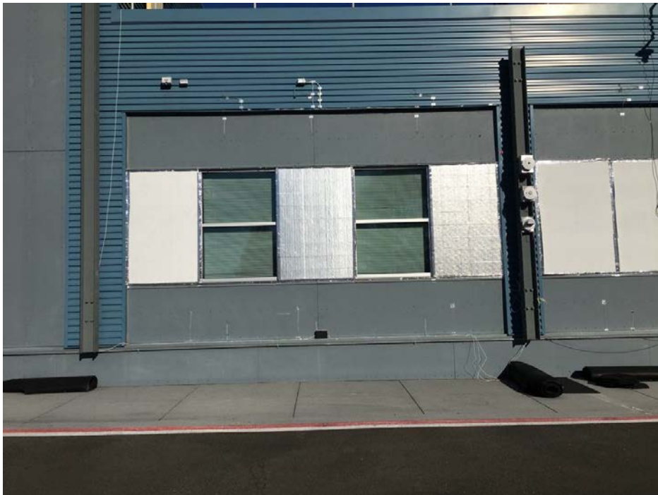
Figure S2. Exterior of cell with foam panels removed from two of five window sections during Classroom experiments.
