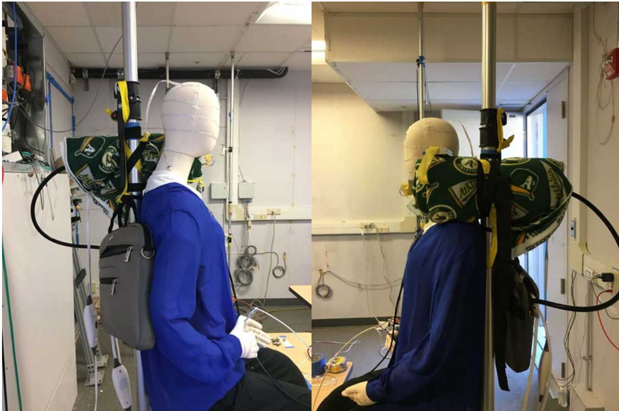
Figure S11. Assembly B with heating pads on supply and at release.
