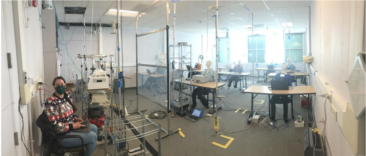
Figure S5. Classroom configuration with release at Teacher position and free-standing barrier placed between Teacher and RIC positions.
