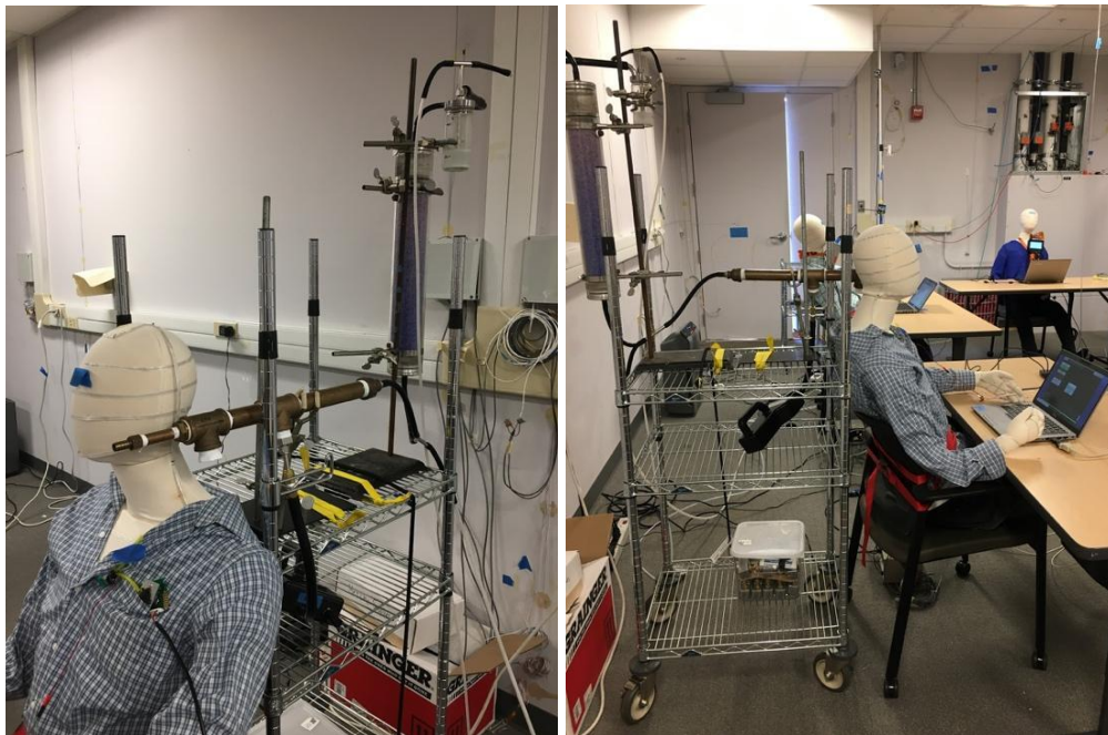
Figure S8. Assembly A configured with Collison nebulizer to release 2 \mu\text{m} PSL particles.
