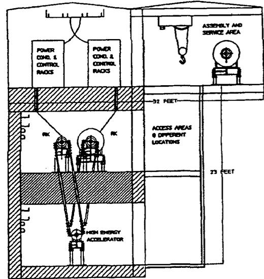
Fig. 8 Elevation view of the RK-TBA accelerator.
