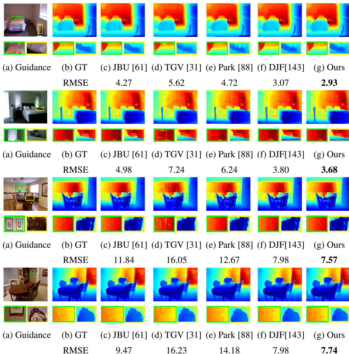
Figure 3.10: Qualitative comparisons on depth upsampling. Comparisons against existing depth upsampling algorithms for a scaling factor of 8\times . The numbers (in centimeter) are the RMSE metric comparing against the GT in (b).
