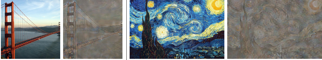
Figure 4.2: Inverting whitened features. We invert the whitened VGG Relu_4_1 feature as an example. Left: original images, Right: inverted results (pixel intensities are rescaled for better visualization). The whitened features still maintain global content structures.
