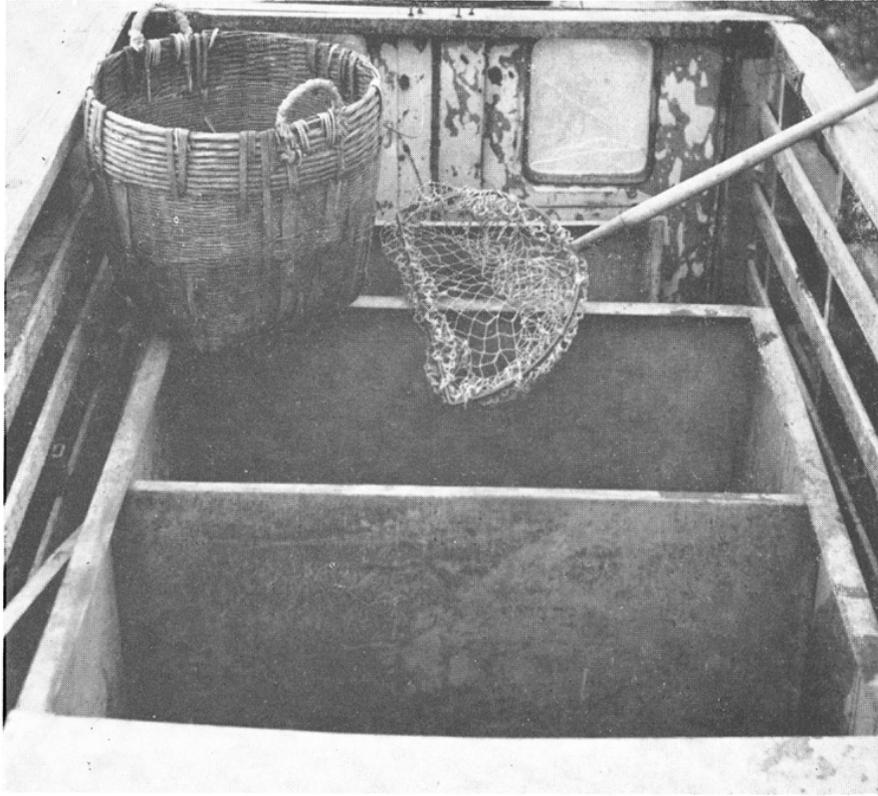
FIGURE 27. Compartments in a rough fish fisherman's tank truck, Sacramento River near Broderick. An aerator supplies oxygen to the water in these compartments when live fish are being transported to market. Note the dip net and fish basket for use in handling the fish. Photograph by Felix A. Miller, December, 1948
