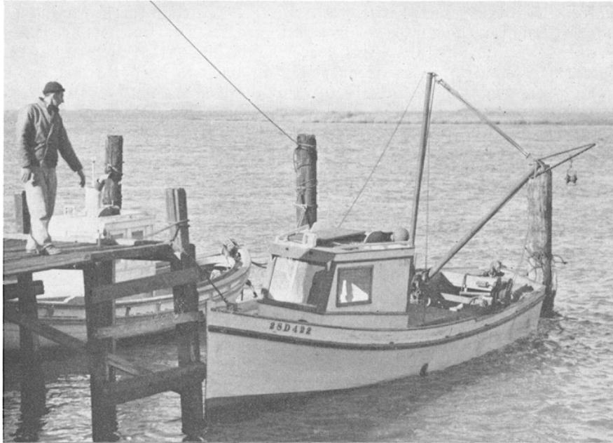
FIGURE 23. A power operated boat with a hoist for handling the large fyke net now in use. Pittsburg, California. Photograph by D. H. Fry, Jr., January, 1949
