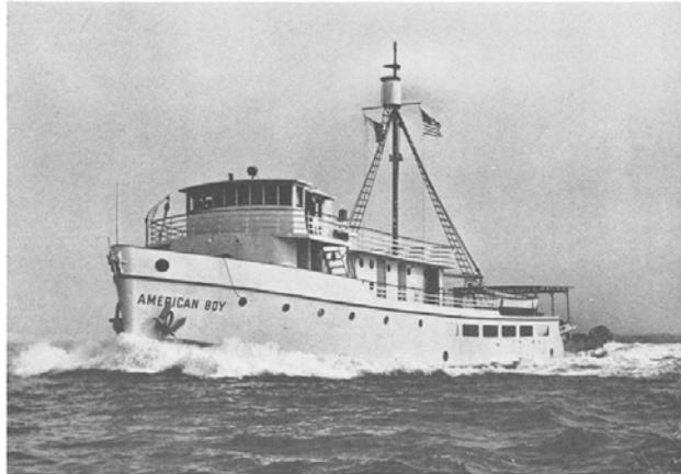
FIGURE 7. A typical modern tuna boat, able to cruise to the equator and back. The entire load of tuna is frozen in chilled brine. Photograph by Kent Hitchcock, Balboa, California, 1947
