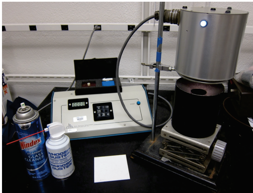
Figure 3. Devices & Services Solar Spectrum Reflectometer, Model SSR-ER, version 6, operated with its measurement head inverted.
