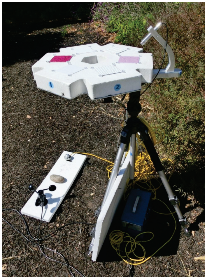
Figure 11: Apparatus for Measurement of Effective Solar Reflectance
