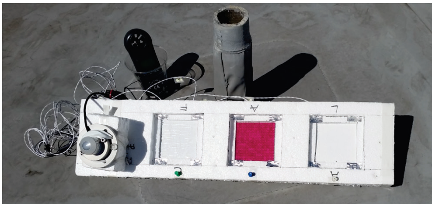
Figure 8. Three-cavity insulated apparatus used to measure the ESA of ruby crystal clear (center cavity). Image also shows the pyranometer and anemometer used to measure solar irradiance and wind speed.
