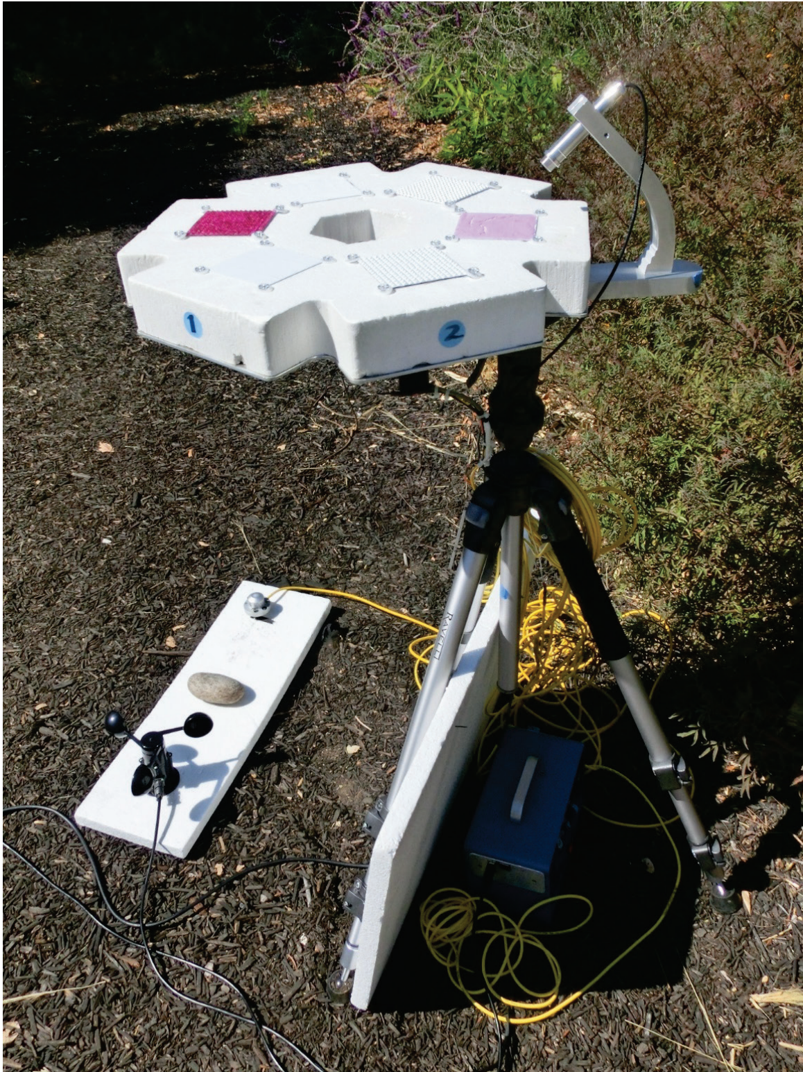
Figure 14. Photo of final apparatus, including rotating platter, IR thermometer (upper right), anemometer (lower left), pyranometer (on same board as anemometer), and control electronics (underneath tripod). The air temperature sensor is hidden below the platter.
