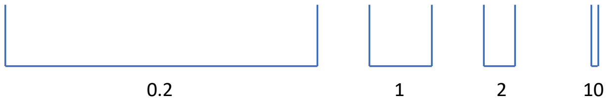
Figure 3. Canyon aspect ratio R = H/W = 0.2, 1, 2, or 10 .
