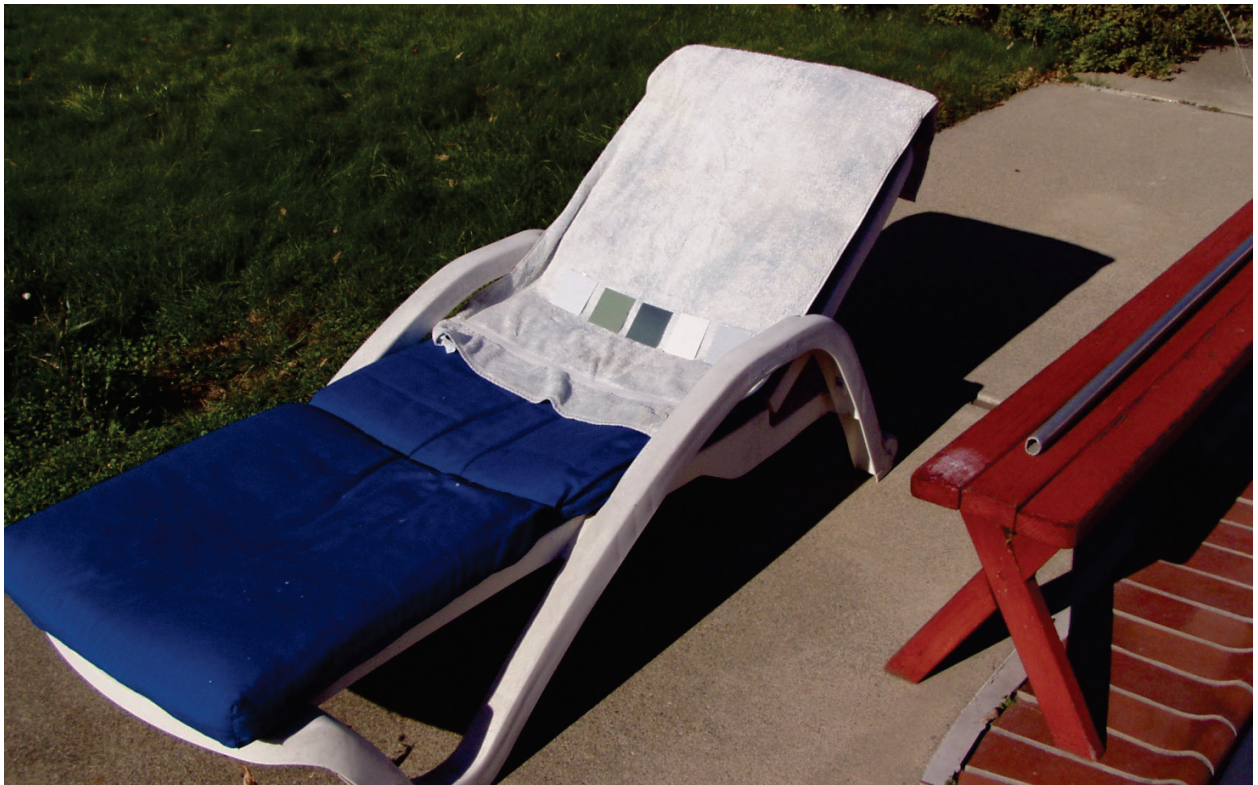
ESM Figure A-3. Reclining chair with towel used to support specimens in Experiment 0. Note that this photo shows a set of specimens different from that used in Experiment 0.
