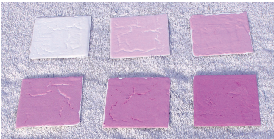
Figure 16: Pink-Red Coatings Incorporating Fluorescent Ruby Pigment
