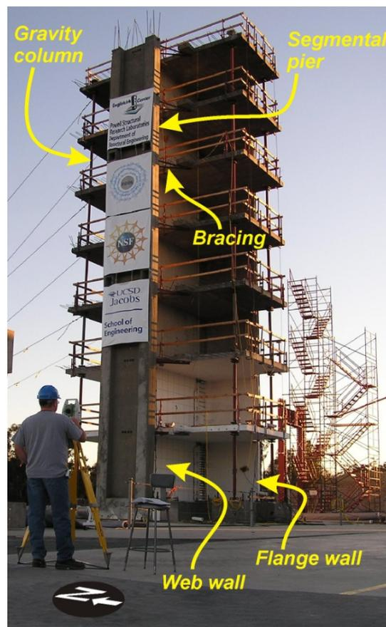
**Fig. 2** Test structure
