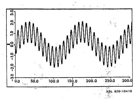
Fig. 1. Electron orbit in wiggle plane, with  $\gamma = 8$ ,  $B_0 = 5$  kG,  $\lambda_W = 5$  cm,  $\frac{dx}{dx}(o) = -0.50$ ,  $a = 1.08 \times 10^{-3}$ ,  $\beta = 6.68 \times 10^{-5}$ , and 30 G/cm dz quadrupole focusing.
