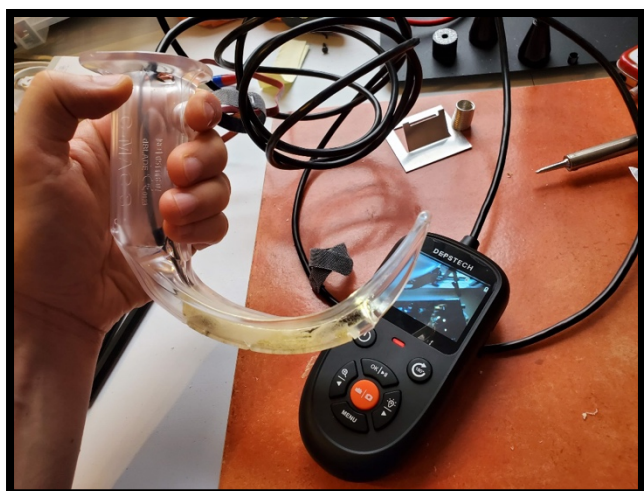
Figure 7: Once the borescope is appropriately positioned and glued within the blade, an expanding foam glue may be used to fill the empty space and stabilize the components.
