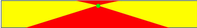
Figure 9: (color online.) Cartoon representation of a hypothetical \beta -particle emission (green circle) that occurs within a fixed solid angle (red areas) towards opposing DSSD (yellow rectangle) hemispheres. The relative average amount of material through which a \beta -particle travels changes depending on the location of the \beta -particle emission, thus affecting the energy-deposition spectrum, as seen in Figure 8.
