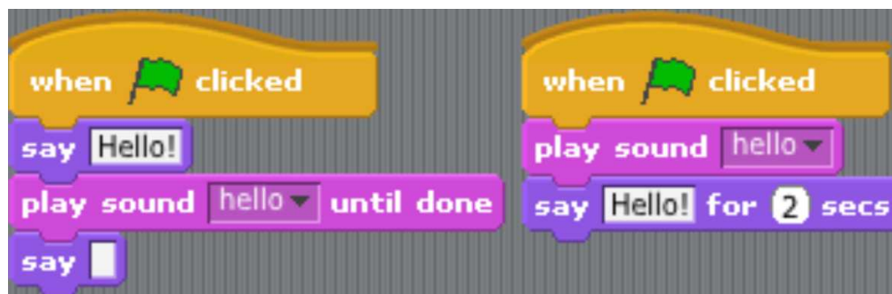
Figure 2.1: Shows the two methods for synchronizing messages from the say MESSAGE blocks with sound files played through the play SOUND blocks. While both methods can produce the desired effect, the method on the right requires manually setting an appropriate duration in the say MESSAGE for SECONDS block and thus is not as robust to modifications, whereas the method on the left guarantees synchronization between the play of the sound file and the display of the message.
