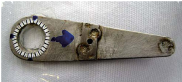
Fig. 2. External fixation device for in vivo OCT and MPM/SHG. 1-mm markings around the periphery provide coordinates for re-localization of lesions at successive imaging sessions. [Figure can be viewed in color online via www.interscience.wiley.com .]
