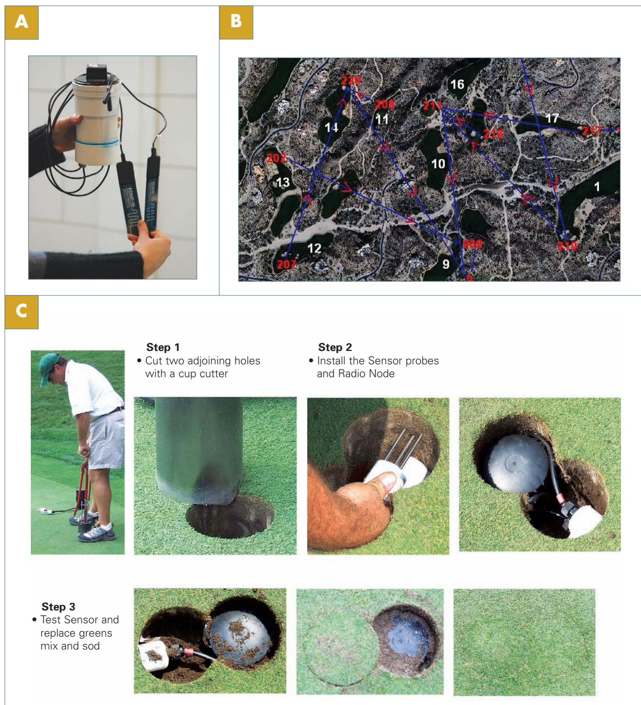
Figure 2.3 Example of static sensors for self-regulating systems. (A) Node with sensor probes for in-ground deployment. Photo: D. Rejeski, WWICS. (B) Communication across golf course mesh network. Image: Advanced Sensor Technology, Inc. (C) Sensors and sensor node installation process on a golf course. Image: Advanced Sensor Technology, Inc.
