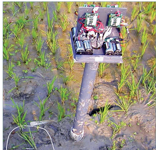
Figure 2.2 Static soil sensor pylon deployed in a Bangladesh Rice Paddy. Rugged PVC enclosures protect communication, power, and computation hardware. Sensors (buried underground) and enclosure cover are not shown. Photo: N. Ramanathan, UCLA.
