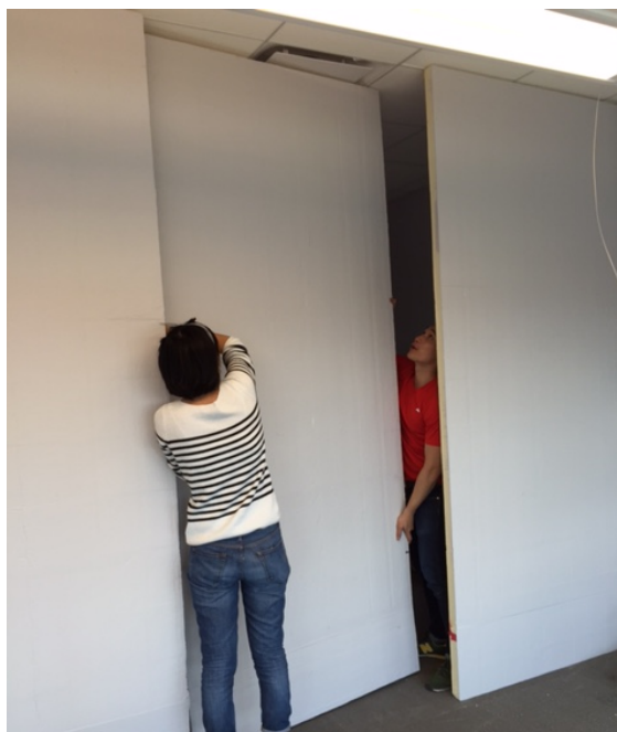
Figure 5. Moveable walls used to change daylight-zone depth.
