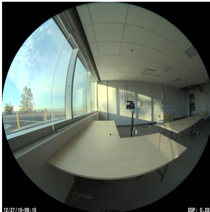
Figure 43. Time-stamped image from an HDR camera set-up positioned perpendicular to the window wall. The calculated DGP for this time is denoted in the lower right corner, and the HDR camera facing the window wall is visible in the center of the image.
