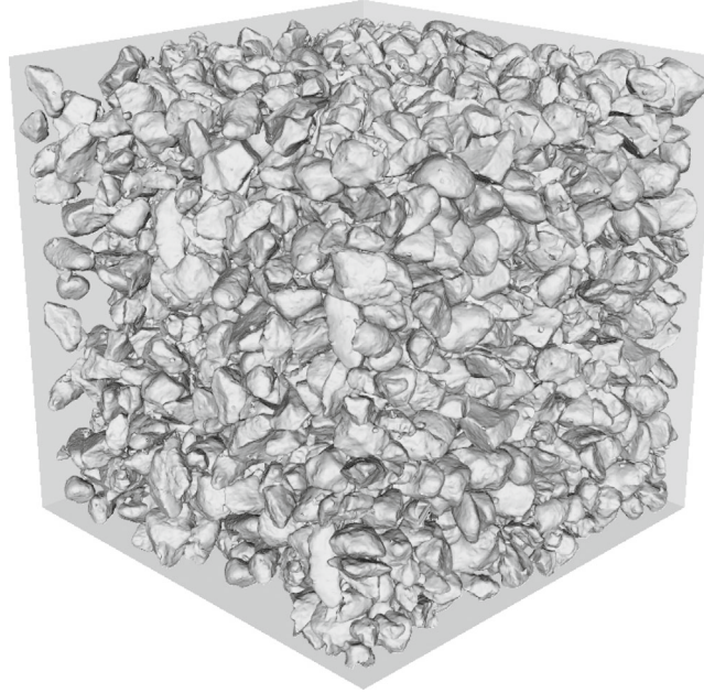
FIGURE 11 Initial configuration of 1600 very high-resolution grains in 800 \times 800 \times 800 domain for impulse-based method with large time steps.
