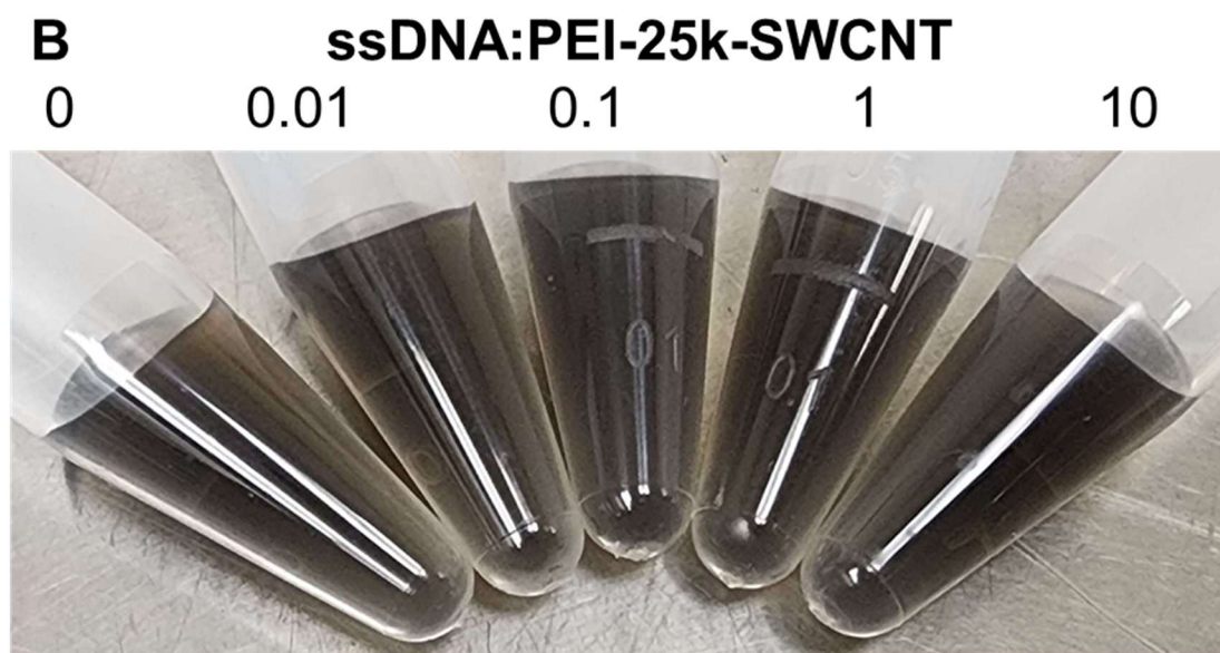
Supplementary Figure 4.3. Aggregation of ssDNA-PEI-SWCNT at high ssDNA:PEI-SWCNT ratio. a) PEI10k-SWCNT visibly aggregated at a 10:1 ratio of ssDNA:PEI-SWCNT, while b) PEI25k-SWCNT did not show any visible signs of aggregation at any of the testing ratios.
