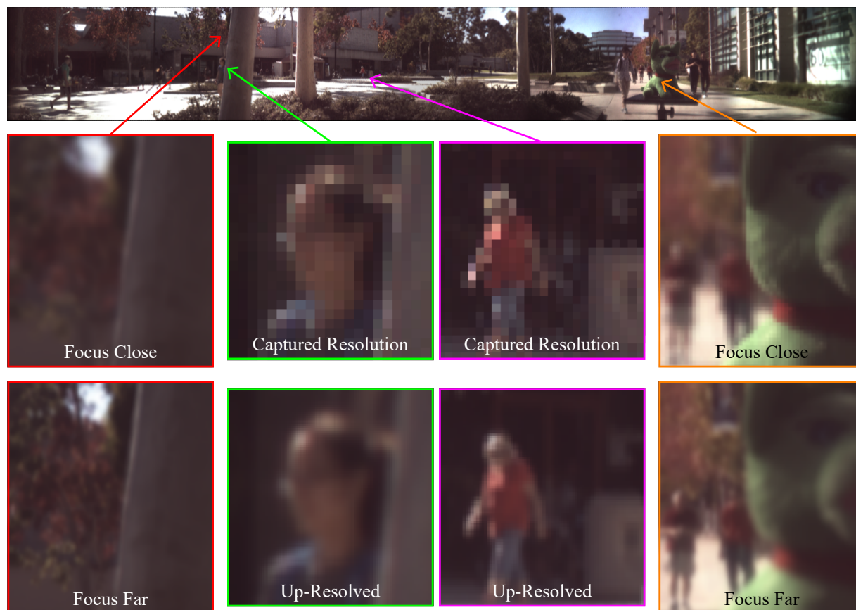
Figure 4.3: Stitched 2D slice (top) of the 138^\circ 72 MPixel ( 15 \times 15 \times 1600 \times 200 ) outdoor LF panorama with zoomed regions showing refocusing and up-resolving.
