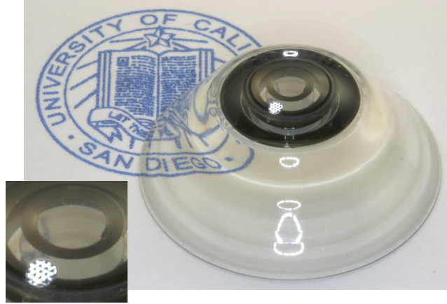
Figure 2.6: Fabricated telescopic contact lens with embedded polarizers and diffusing retroreflector. The inset shows the retroreflector illuminated by a ring light around the camera and seemingly suspended fourth mirror.
