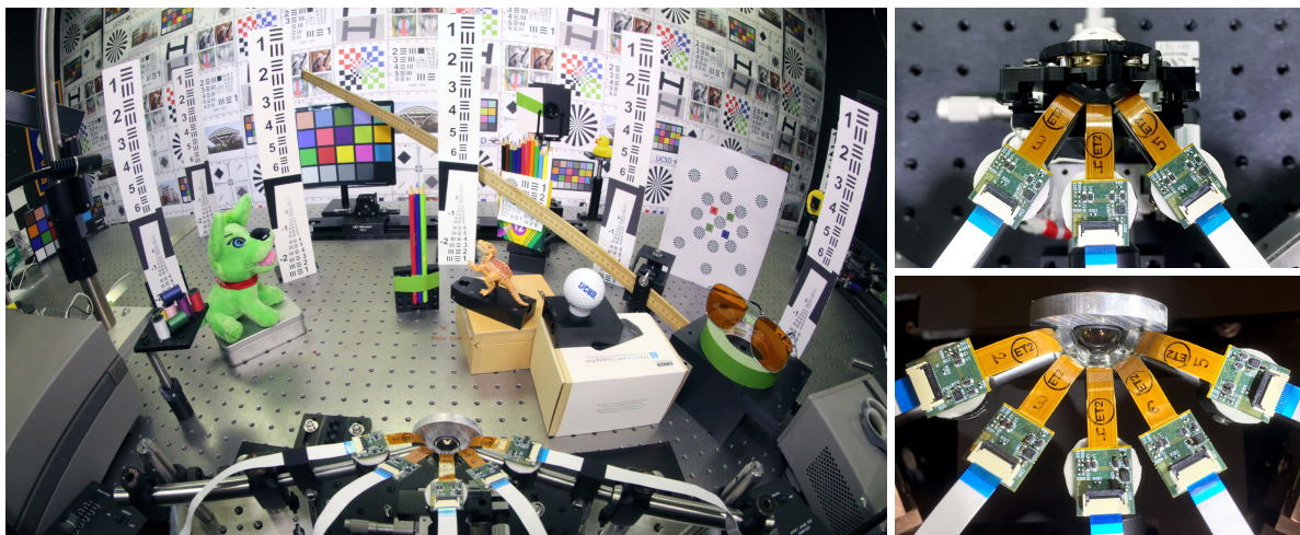
Figure 4.18: Photo of lab scene with fish-eye lens (left), F/2.5 three sensor camera (top right), and F/4 five sensor camera (bottom right).
