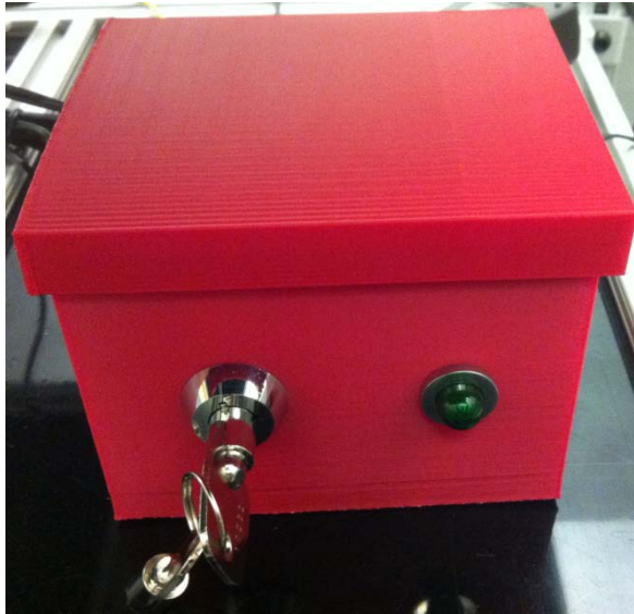
Figure 7 Photograph of interlock box
