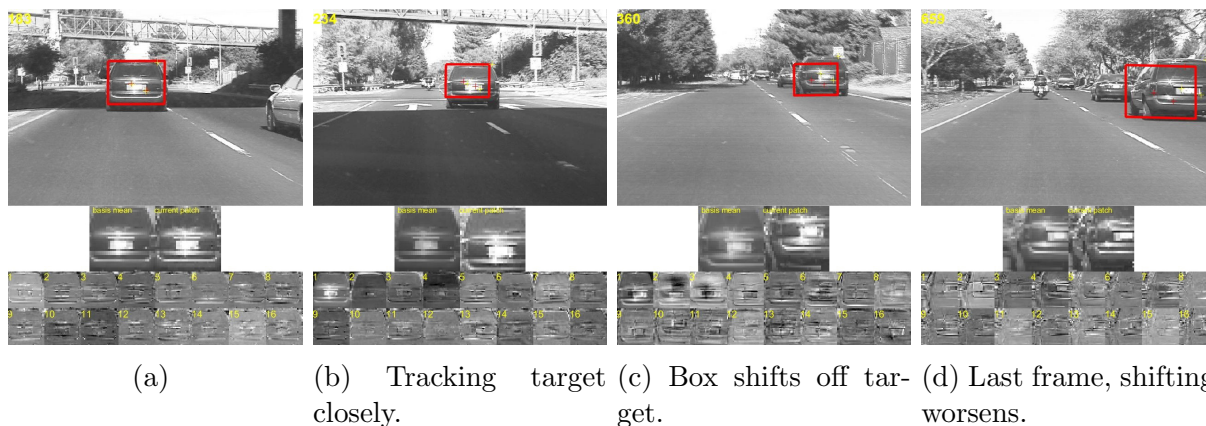
Figure 3.28: The key video frames of the modified IVT tracking performance of video “car4.” The video frame is shown with the target feature to be tracked (marked by a yellow cross), the estimated target feature location (marked by a red cross) and the image patch (a red frame). The reference image patch is shown below the video frame on the left, while the currently selected image patch is on the right. Below the image patches are the dictionary templates and beneath the templates is the weighting of each templates.
