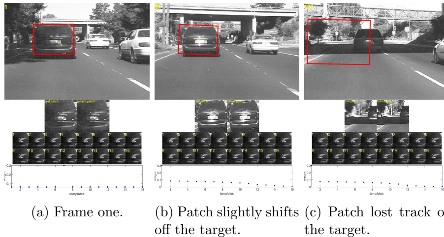
Figure 3.9: The key video frames of the RVT tracking performance of video “car4” based on the proposal of Mei et al. The video frame is shown with the target features to be tracked as the ground truth (marked by the yellow crosses), the estimated target feature location (marked by a red cross) and the image boundary box estimate (a red frame). The chosen image patch is shown below the video frame on the left, while the currently selected image patch is on the right. The dictionary is shown at the beneath the image patches, where each template is displayed. Below the dictionary is the weighting of each templates.
