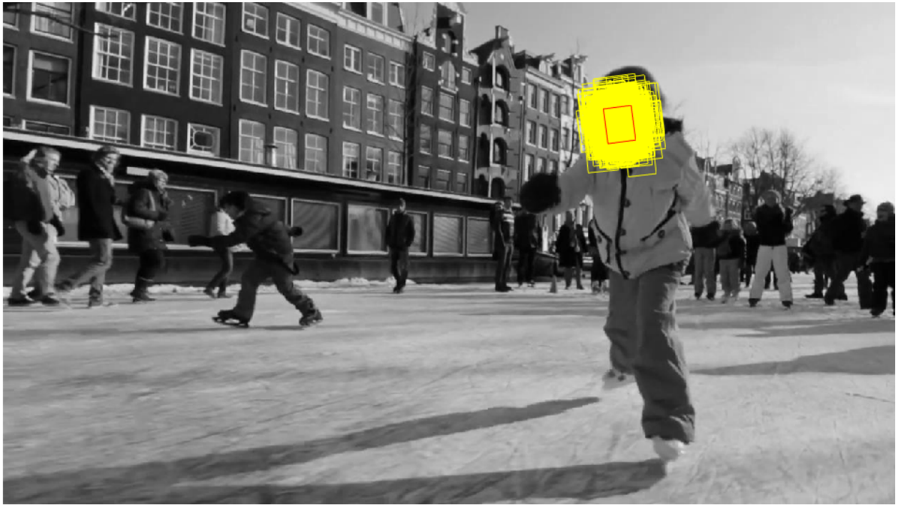
Figure D.2: The example illustration of the target boundary boxes of the particles drawn (yellow boxes) and the estimated target boundary box of the previous frame (red box).
