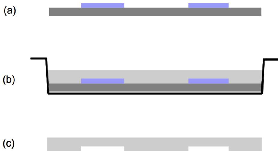
Figure 5.19: Fabrication of the PDMS fluid channels. (a) The initial step is to produce the mold on a Si wafer. The Si wafer must undergo a passivation with Sigmacote before applying PDMS. (b) The mold was fixed to the bottom of a petri dish and PDMS solution was poured on to the mold. PDMS was baked in a 65 °C oven after degassing to remove air bubbles. (c) Peel off the PDMS layer from the wafer.
