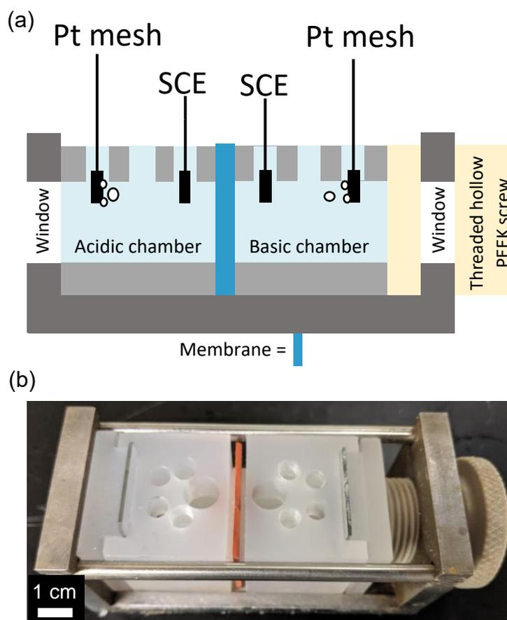
**Figure 2.** (a) Diagram of the electrochemical H-cell indicating the general placement of the electrodes and the membrane. (b) Digital photograph of a dry electrochemical cell incorporating a red silicone sheet to indicate where the membrane would be located and where the largest holes are 1 cm in diameter.
