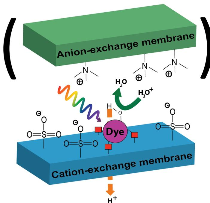
**Figure 1.** Diagram representing a photoacid-sensitized cation-exchange membrane. Our data are consistent with a process where upon absorption of light the photoacid dye releases a proton that then transports through the cation-exchange membrane. Addition of an anion-exchange membrane to form a bipolar membrane structure resulted in a significantly larger photovoltage.
