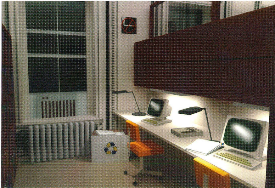
Figure 8. A rendering from the RADIANCE computer simulation program showing a simulation of how a cubicle in the Office of Environmental Policy (OEP) suite would look under one of the design scenarios considered.
