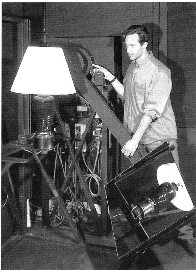
Figure 6. Researcher checks the alignment of LBL's recently completed mirror-based goniophotometer. A goniophotometer is used to measure the angular distribution of light (candlepower) emanating from a lighting fixture.
