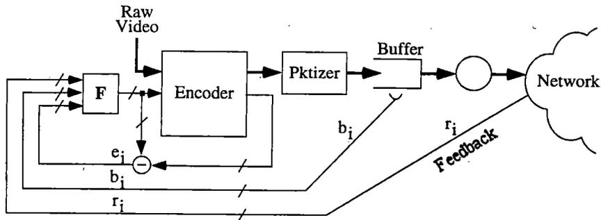
Figure 2: Video encoder and rate controller
