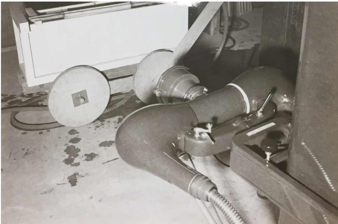
Figure 1.3. X-ray tube and moveable tank used for irradiating fish in the canvas retaining sling. Source: UWFL-1, “Equipment and Procedures used in Irradiation of Fish with X-Rays.” UWLRB, Box 9, Volume 1, Figure 2. University of Washington Libraries, Special Collections, Laboratory of Radiation Biology records. Accession no. 00-065. Republished with permission of University of Washington Libraries.
