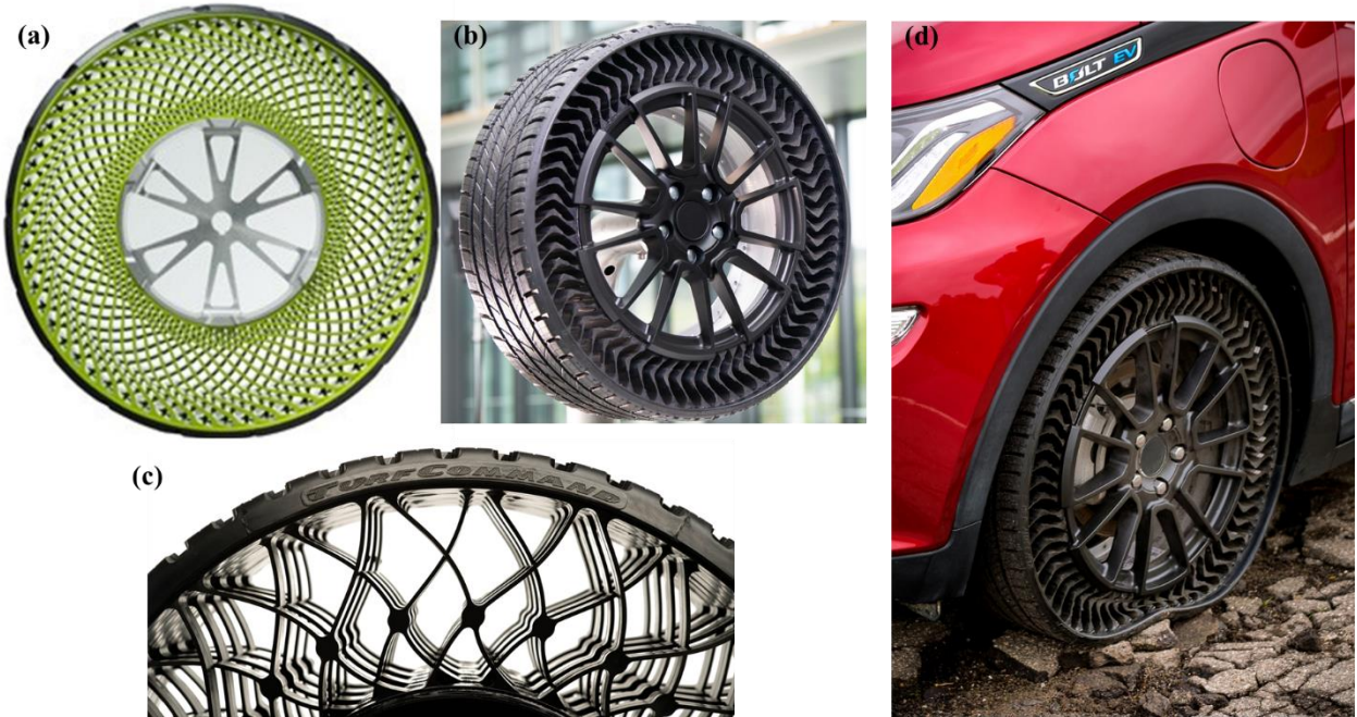
Figure 4.3: Different airless tire concepts from commercial companies. (a) Bridgestone airless tire [201]; (b) Michelin airless tire [202]; (c) Goodyear Turf Command airless tire [200]; (d) Michelin airless tire on a real EV [199].
