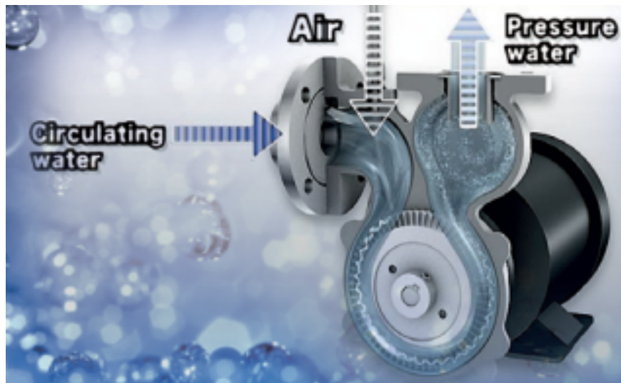
Figure 2.5: Schematic of the Nikuni Micro-Nano bubble generator
