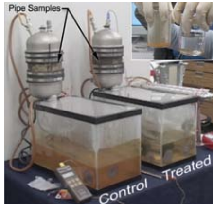
Figure 1.4: Photograph of the test systems with the mild steel pipe samples from Three Mile Island Nuclear Power Station.
