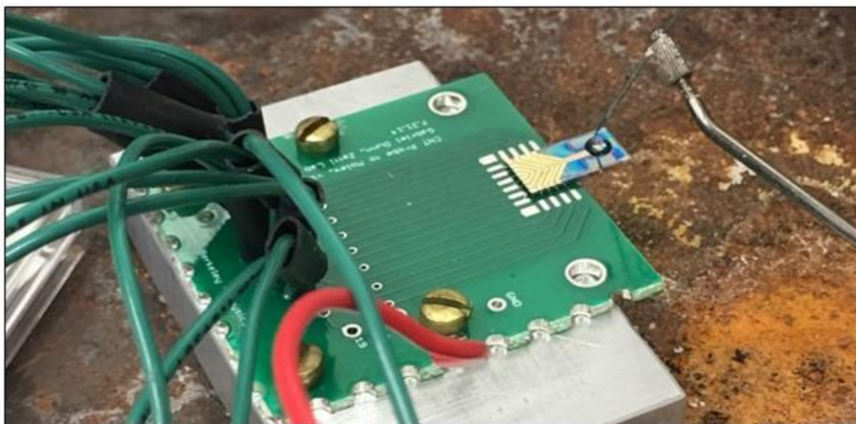
Figure 5.21: Electrochemical Test Setup for Multi-Unit Array. EIS was performed using a platinum counter electrode. The backplane of the Si-chip and PCB were at a common ground with the counter electrode. Dulbecco phosphate buffer solution (DPBS) – a biological buffer solution – was used as the solution.
