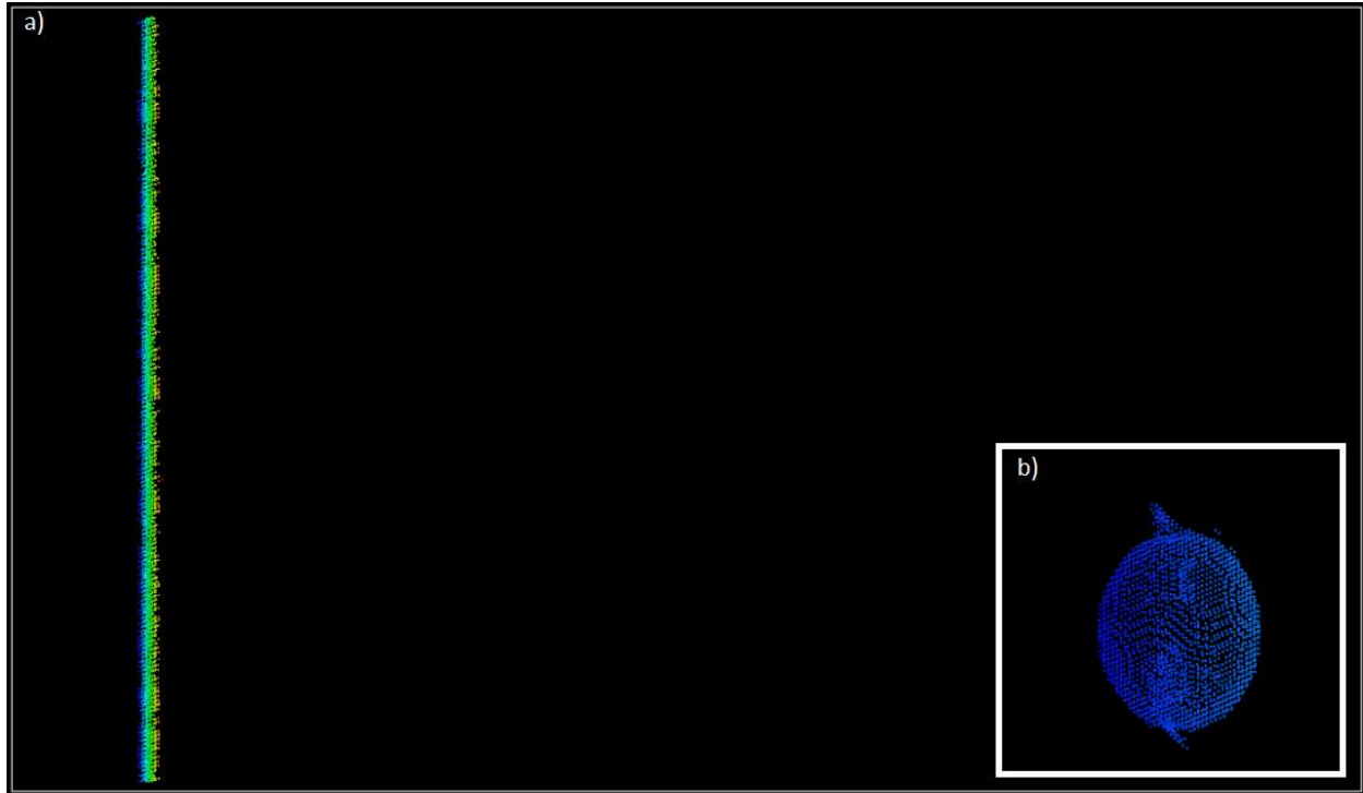
Figure 5-8 54 GPa (2 km/s piston velocity) simulation for [111] diamond shock at 10 ps. a) A view of all atoms within the system with coordination number other than 4, the usual value for diamond. No atoms beyond the piston surface are detected, i.e., all are diamond. b) The beginnings of dislocations can be seen to form when a void is present and shocked, but never begin to propagate within the system.
