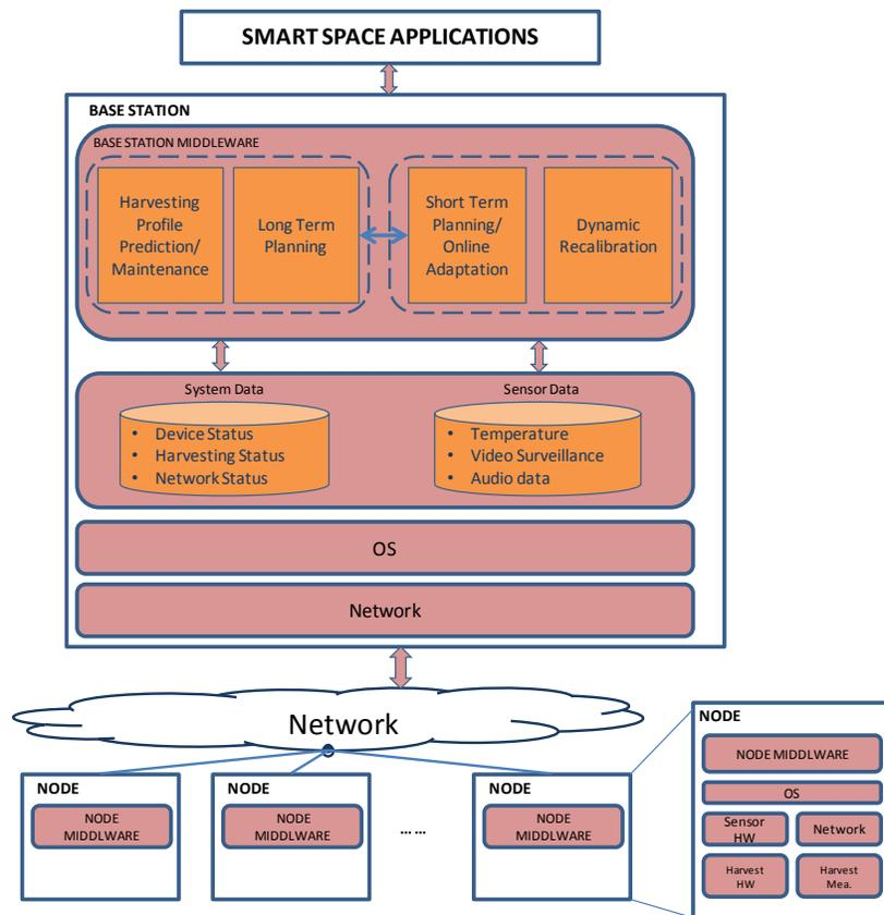
Figure 2.3 Architecture of an Energy Harvesting Network
