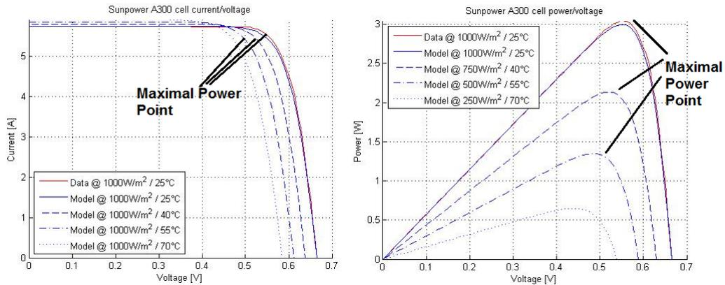
**Figure 2.2 I-V Characteristics of an Example Solar Cell**
