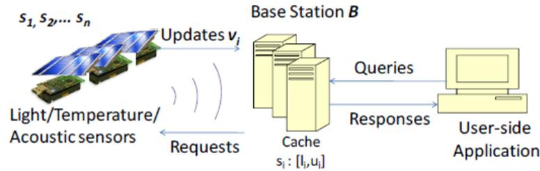
**Figure 3.1 Data Collection in Wireless Sensor Networks**
