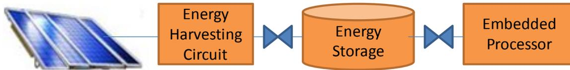
**Figure 1.1 Solar-Powered Embedded Systems**
