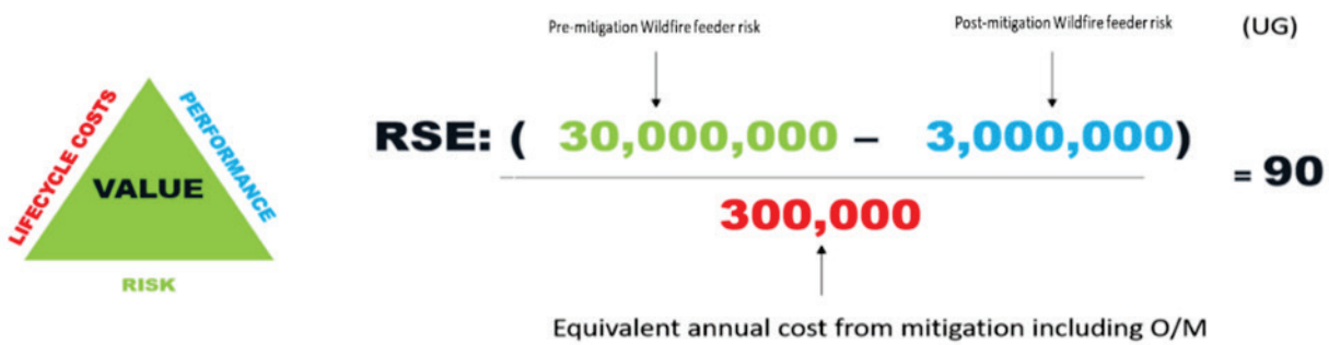
Figure 8.4. Illustrative Risk-Spend Efficiency Assessment for Undergrounding
