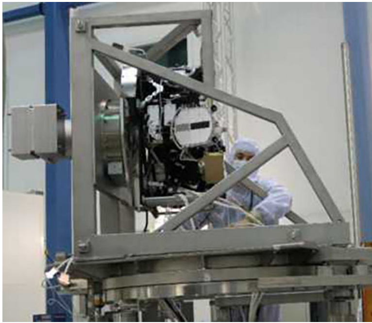
Figure 16. ICON FUV mounted on its side on the articulating cradle inside the vacuum chamber. Turret and contamination cover door are nearest to the reader.
