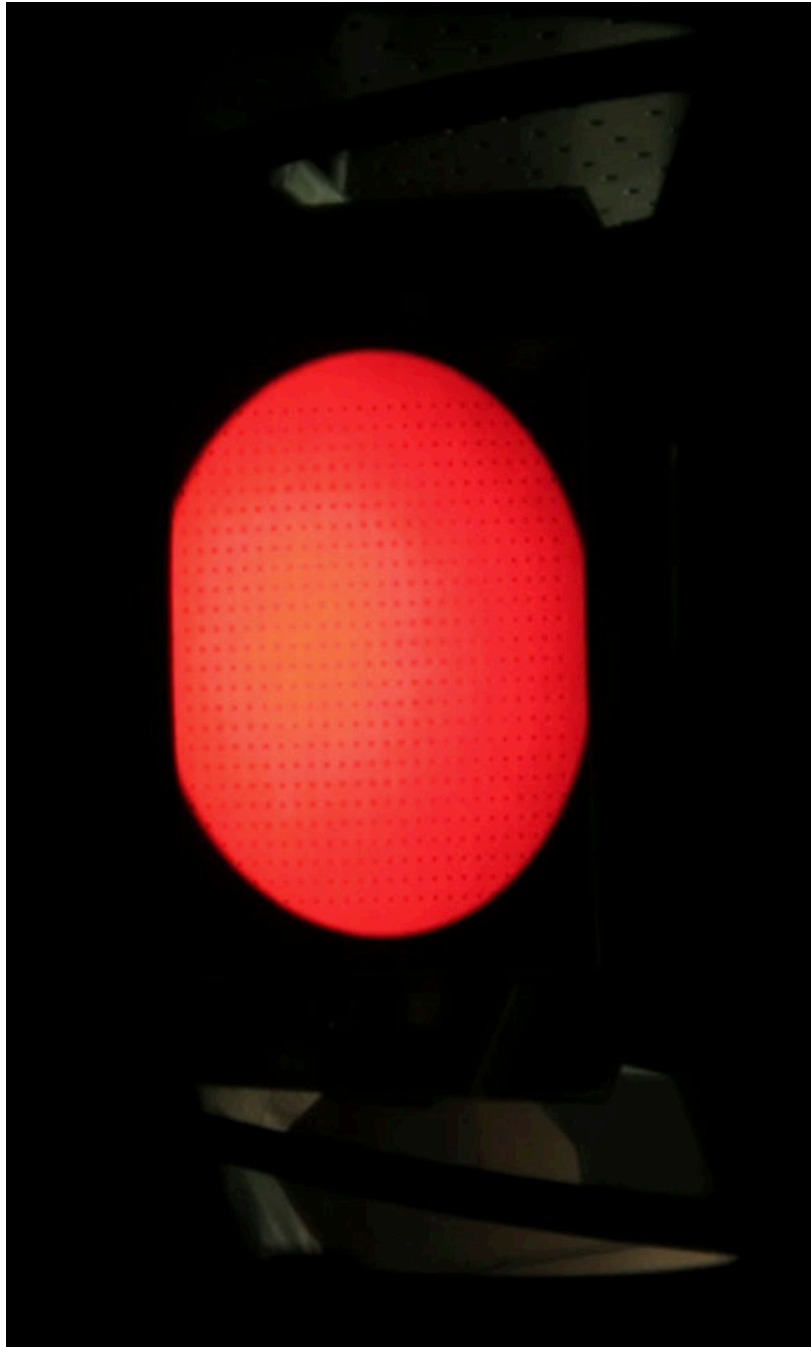
Figure 14. LW channel image of a test pattern illuminated with 628 nm light while the non-flight 900 lines/mm grating was installed in ICON FUV.
