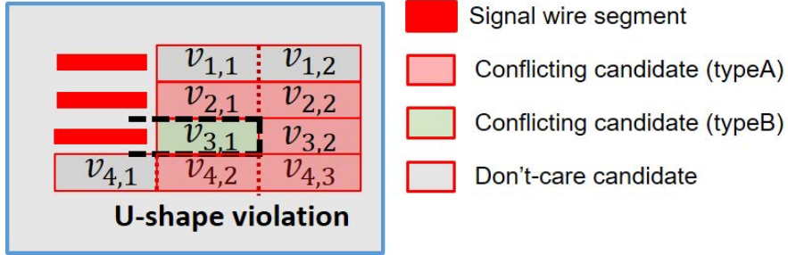
Figure 2.8: Illustration of a U-shape block mask rule violation.
