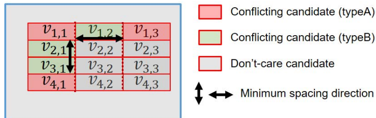
Figure 2.13: Illustration of conflict list enumeration for minimum spacing constraint, showing horizontally and vertically conflicting pairs.
