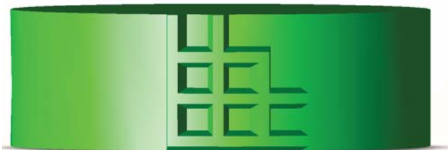
Figure 8: Solid Model of Roll with Raised Patterns
