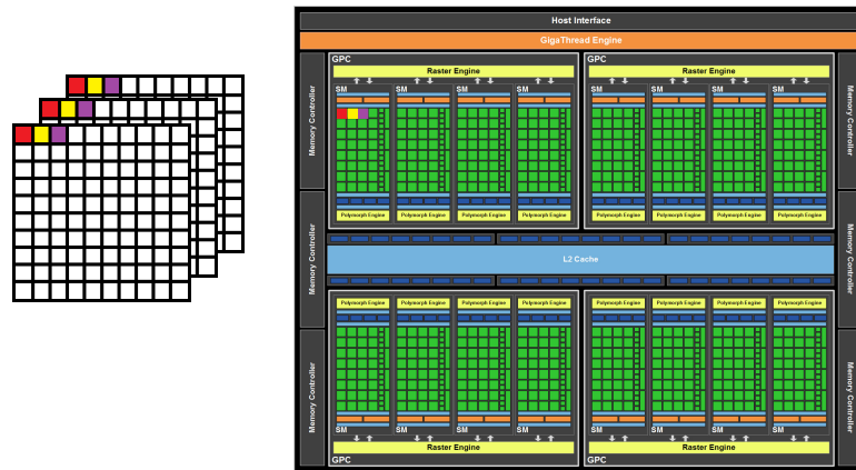
Figure 3.3: To perform the interpolation and reparametrization steps of the string method, each grid point is assigned to a single thread, and each thread runs on a single GPU core.
